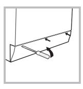
3. Remove the covering panel on the front of the washing machine using a screwdriver (see figure).
