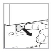
4. Using the tab shown in the figure, pull outwards until the plastic brace comes away; pull it downwards until you hear a "click", which indicates that the door is unlocked.
