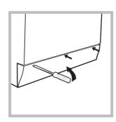
1. Remove the covering panel on the front of the machine using a screwdriver (see figure).
