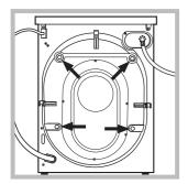
2. Remove the four protective screws and the rubber bush with the respective spacer, situated on the rear of the appliance.
