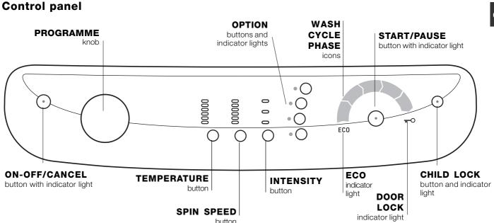
**ON-OFF/CANCEL** button with indicator light  $\circlearrowleft$ : press the button briefly to switch the machine on or off. The green indicator light shows that the machine is switched on. To switch the washing machine off during a wash cycle, press and hold the button for approximately 2 seconds; pressing the button quickly or accidentally will not switch the machine off. If the machine is switched off during a wash cycle, the programme will be cancelled.
