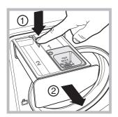
To remove the drawer, press the lever (1) and pull it outwards (2) (see figure).
