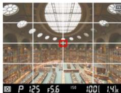
**Virtual horizon:** Alternatively, the **Info** button can be used to display pitch and roll indicators to help you keep the camera level during live view.
