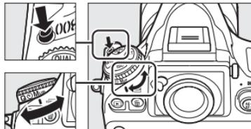
After focusing, press the shutter-release button all the way down once to raise the mirror and again to release the shutter. An optional remote cord can be used to prevent the camera moving when you press the shutter-release button, or you can select an option other than **Off** for Custom Setting d4 (**Exposure delay mode**) to delay shutter release until about 1–3 s after the button is pressed. Use of a tripod is recommended.
