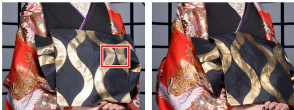
The photo on the left was taken with the D800E, that on the right with the D800. Color artifacts are visible in the sash.
