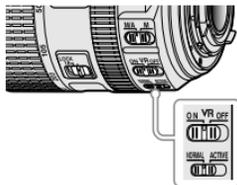
If the lens has a vibration mode switch, choose **NORMAL** for hand-held photography or when using a monopod. Vibration reduction should generally be turned off when the camera is on a tripod (exceptions can be made for the AF-S NIKKOR 200mm f/2G ED VR II and other lenses with a **TRIPOD** option).
