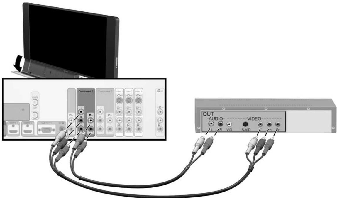
**NOTE:** You can connect to the Component 1 and Component 2 inputs on the TV.
