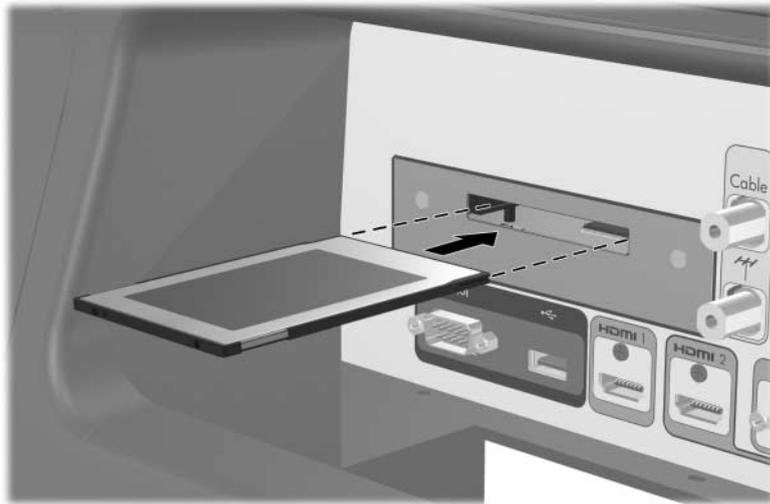
2. Gently push the card into the slot until it stops. When fully inserted, the card sticks out of the slot.
