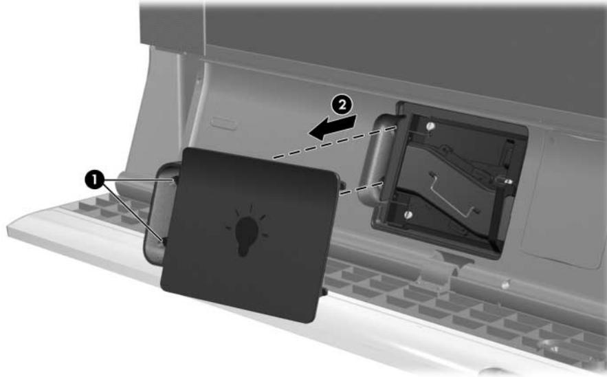
5. Loosen the three screws ❶ on the lamp module; then pull out the module using its handle ❷.
