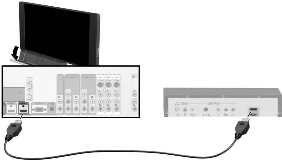
**NOTE:** You can connect to the HDMI 1 and HDMI 2 inputs on the TV. The HDMI cable carries both the video and audio signals.
