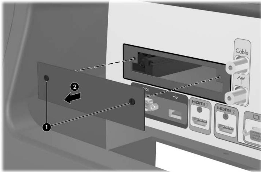
4. Insert the CableCARD module ❶ into the opening and firmly press it into place until the front plate is flush with the panel.
