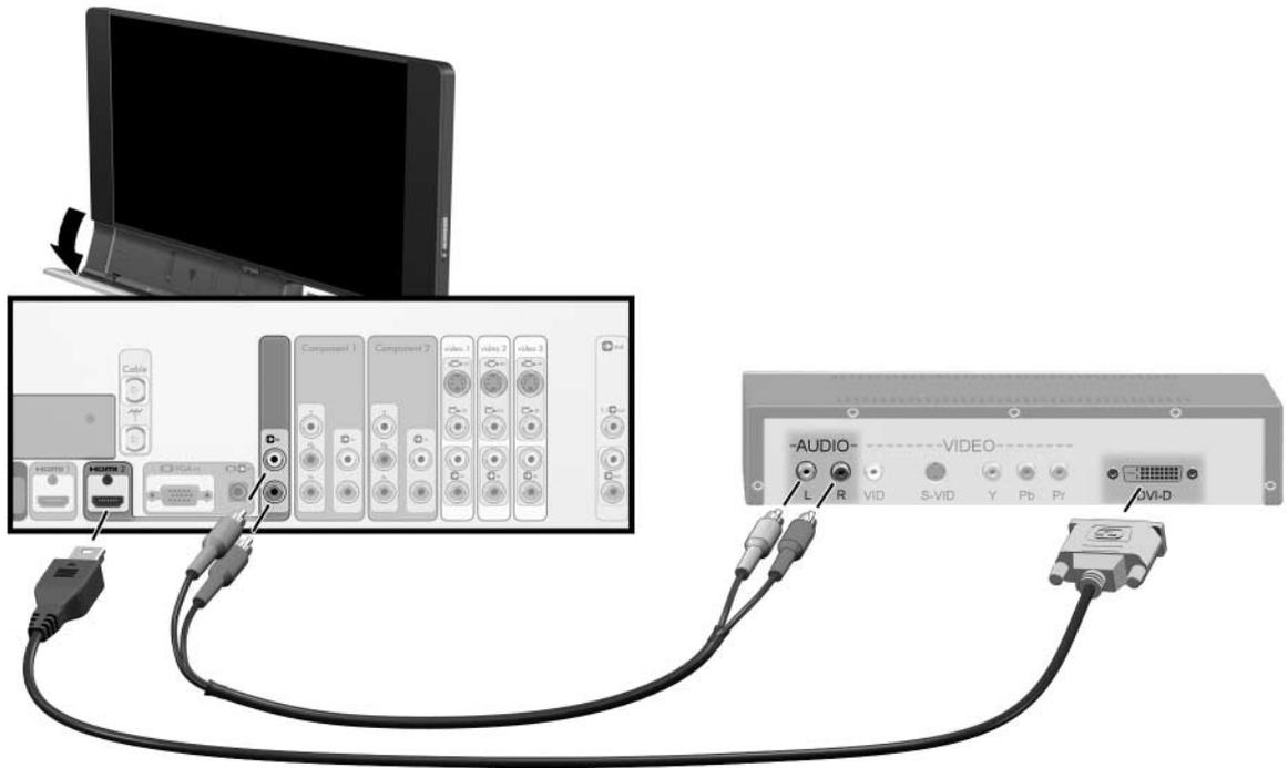
**NOTE:** If you are using the TV speakers, connect a DVI device only to the HDMI 2 input on the TV. If you are connecting audio directly to a sound system, you can connect DVI devices to the HDMI 1 and HDMI 2 inputs.
