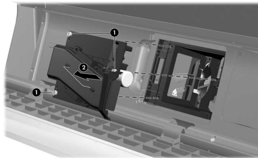
6. Insert the new lamp module into the opening, firmly press it into place, and tighten the three screws ①.
