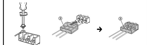
Pass the wires through the cap, connect the wires, then cover the terminals with the cap.
