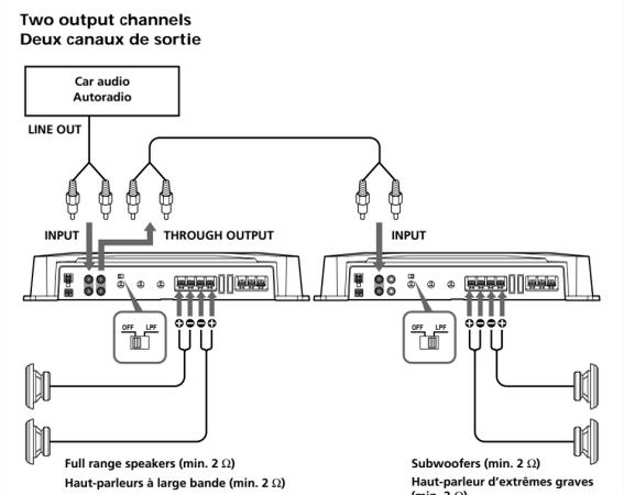
Use the THROUGH OUTPUT terminal when you install more amplifiers. The signals are output as they were input. (LOW BOOST, LPF do not work.)
