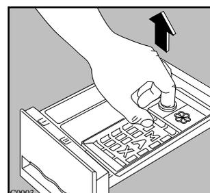
Detergent can also eventually accumulate inside the drawer recess: clean it with an old toothbrush. Refit the drawer after cleaning.
