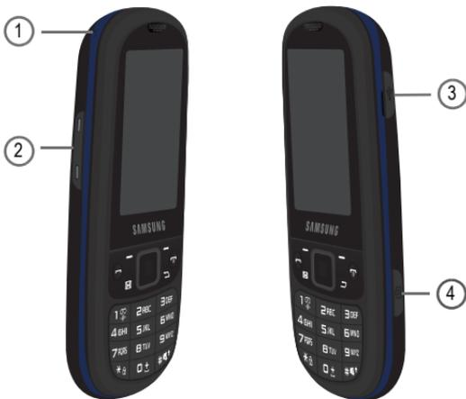
1. **Phone anchor** allows you to connect a strap with which to carry the phone. Remove the back battery cover to fully install a strap to this phone anchor.
