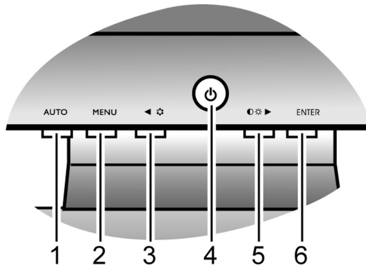
1. "AUTO": Adjust vertical position, phase, horizontal position and pixel clock automatically.
