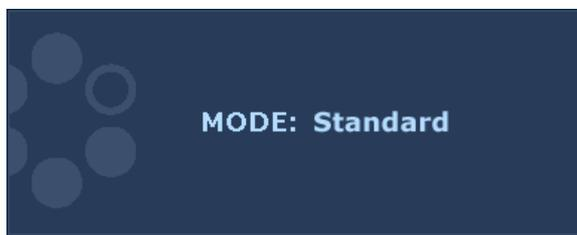
Press the **◀** key continually to switch between the 5 modes for the main window, including **Standard**, **Movie**, **Dynamics**, **Photo**, and **sRGB**. The setting will take effect immediately.
