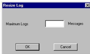
**Note:** “Maximum logs” refers to the number of text lines, or messages, maintained by the Meridian Digital Telephone IP Adapter unit. The Meridian Digital Telephone IP Adapter unit currently retains a maximum of 1000 text lines.
