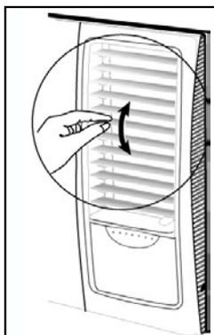
Airflow direction adjustment Up-and-Down.
