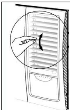
Airflow direction adjustment Up-and-Down.
