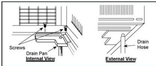
4. Connect the drain hose to the outlet of Drain Pan bottom.
