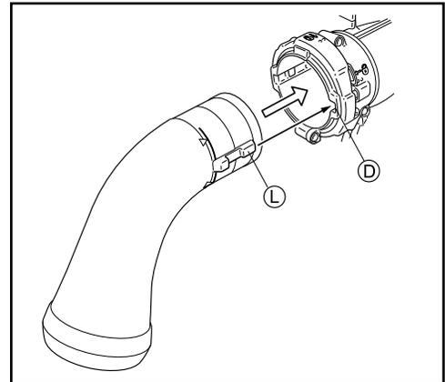
4. After inserting elbow into fan case so that line (M) meets locking ring (C), rotate locking ring clockwise 1/8 turn to lock elbow in place.
