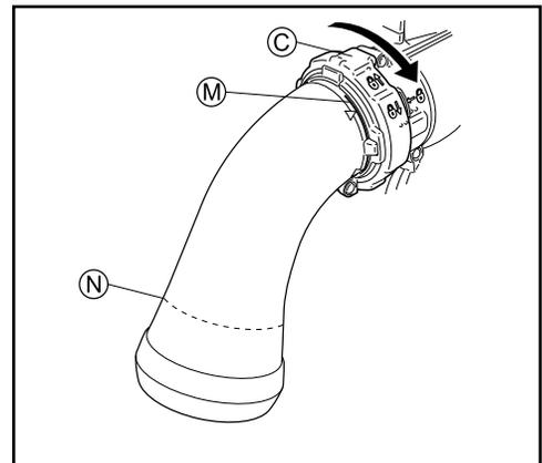
5. Place debris bag opening over flared end of elbow, and cinch bag (O) securely at the position (N) with Velcro strap.
