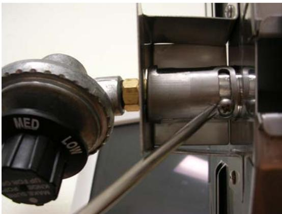
To adjust for proper flame, use a Philips screw driver to loosen screw. Turn clockwise to close the air shutter, and counterclockwise to open. After adjusting, tighten screw to fix air shutter.
