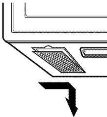
2. Soak grease filter in hot water and a mild detergent. Rinse well and shake to dry. Do not use ammonia or place in a dishwasher. The aluminum will darken.
