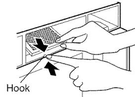
6. Slide a new charcoal filter into place and close the door. The filter should rest at the angle shown.
