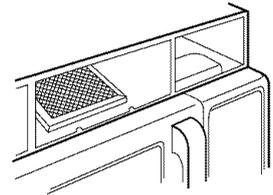
7. Slide the bottom of the vent cover into place. Push the top until it snaps into place. Replace the mounting screws. Turn the power back on at the main power supply and set the clock.
