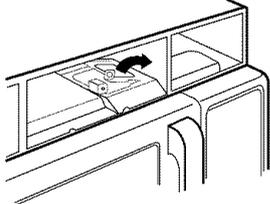
5. Replace bulb with a 30 watt appliance bulb.
