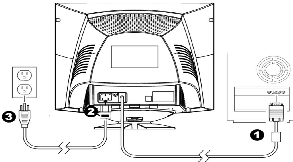
1. Connect the built-in video cable into the 15-pin connector on the back of your computer and tighten the two screws.
