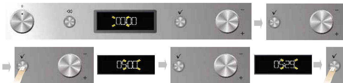
After setting the language, the time must be set on the clock. The two hour digits flash on the display.
