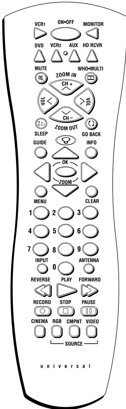
**ANTENNA** When the remote is in HD RCVR mode, switches the HD receiver between Antenna A and Antenna B.
