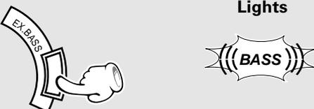
÷ Each press switches EX.BASS on and off alternately.
