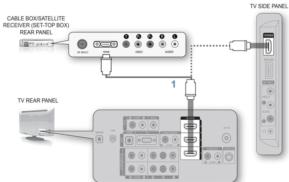
1. Connect an HDMI Cable (Not supplied) between the **HDMI IN (1, 2, 3 or 4)** jack on the TV and the HDMI jack on the Cable Box/Satellite receiver (Set-Top Box).
