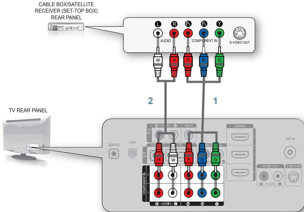
1. Connect a Component Cable (Not supplied) between the **COMPONENT IN (1 or 2) [Y, P<sub>B</sub>, P<sub>R</sub>]** jacks on the TV and the **COMPONENT** jacks on the Cable Box/Satellite receiver (Set-Top Box).
