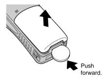
Replace the battery. Then place the battery leads inside the groove, otherwise the leads may be damaged when closing the cover.
