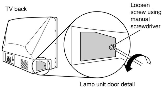
4. Using a manual screwdriver, loosen the two screws on the lamp unit.
