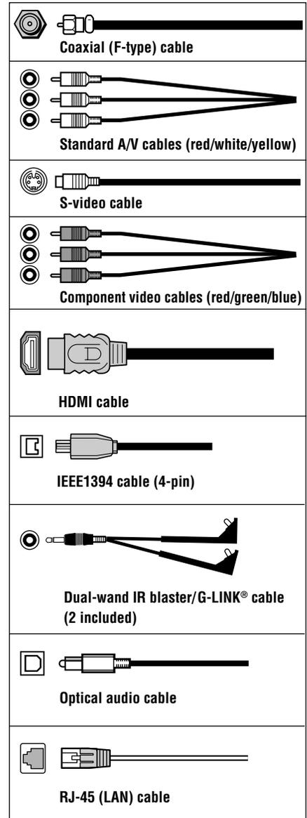
**Note:** Although your TV includes both HDMI and IEEE1394 connections, it may not operate with another device you have that includes such a connection. For example, the IEEE1394 ports are not intended to operate with current model Mini DV camcorders, and the HDMI input is not intended for connection to a computer. Copyright protection requirements may also prohibit or limit connectivity. See page 19 for details about the HDMI input. See pages 22–24 for details about the IEEE1394 ports.
