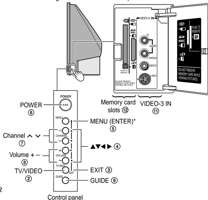
\* The MENU button on the TV control panel functions as the ENTER button when a menu is on-screen.
