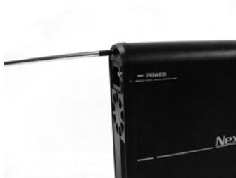
Note: When removing the 5.25" device from the Nexstar DX, be careful not to yank on the SATA cable or the power cable. To remove the SATA cable, grasp the cable between your thumb and index finger and gently pull at the sides until the cable comes loose. To remove the power cable, grasp the sides of the plug and pull.
