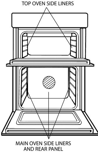
The surfaces of the oven liners are treated with a special vitreous enamel which absorbs cooking soils. At temperatures of 220°C (425°F) or above, the special surface enables these soils to be slowly destroyed. The higher the temperature the more effective it is.
