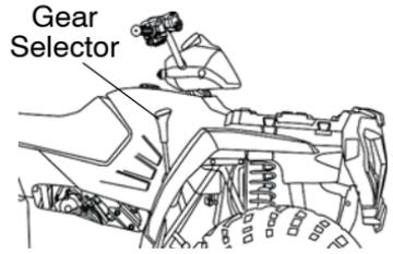
To shift gears, brake to a complete stop. When the engine is idling, move the lever to the desired gear.
