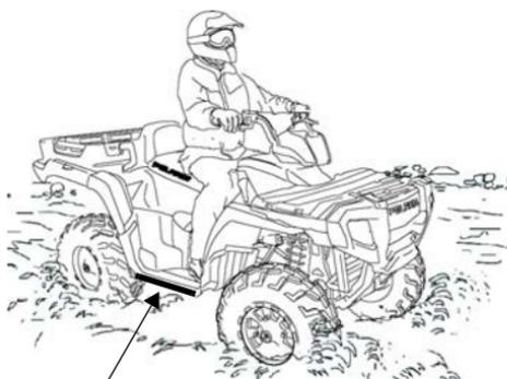
**NOTICE:** Major engine damage can result if the vehicle is not thoroughly inspected after operation in water. Perform the services outlined in the maintenance chart. See page 75. The following areas need special attention: engine oil, transmission oil, demand drive fluid and all grease fittings.
