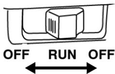
Both the main switch and the engine stop switch will shut off all electrical power to the vehicle, including lights.
