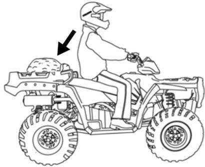
1. Always load the cargo box with the load as far forward as possible.
