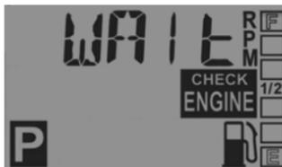
*Example:* For the two blink codes 42 and 36, the Check Engine icon will flash 4 times, pause, then flash 2 times (code 42), then pause longer, blink 3 times, pause, and blink 6 times (code 36).
