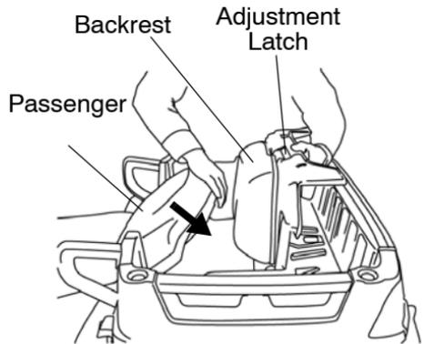
8. To return the vehicle to single-rider operation, reverse all steps. Always lower the passenger backrest to the lowest position before folding it down into the cargo box. Turn the operator backrest latches 1/4 turn to secure the locks.
