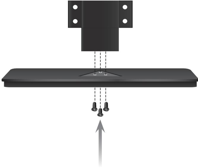
Align the neck with the base and snap it into place.
