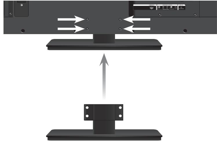
Align the neck piece with the slot in the bottom of the TV and slide it into place as shown.
