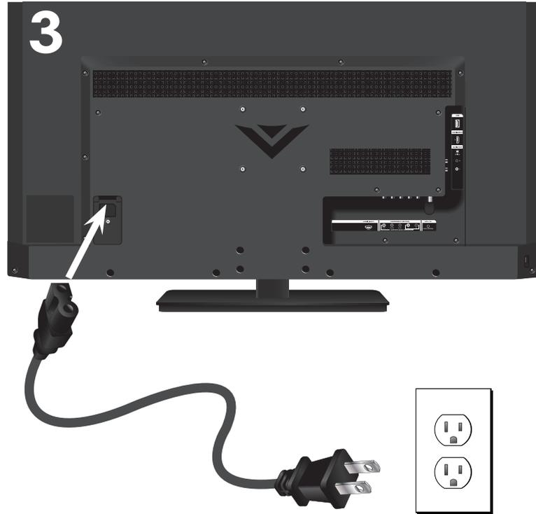
Connect the power cord to the back of the TV. The flat edge of the connector goes toward the outside of the TV.
