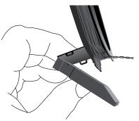
Push the tab into the open slot in the base of the stand. Press until the tab clicks home.
