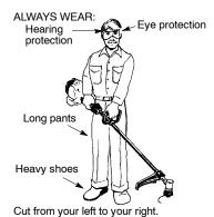
**AWARNING:** Always wear eye protection and hearing protection. Never lean over the trimmer head. Rocks or debris can ricochet or be thrown into eyes and face and cause blindness or other serious injury.
