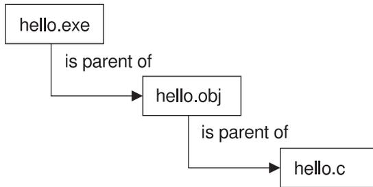
*Figure 45. The build tree for the hello application*
