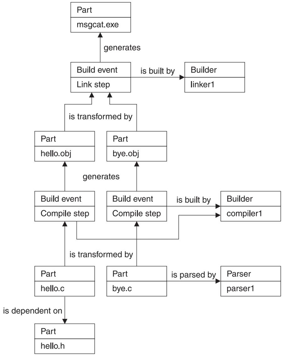
Figure 44. Sample build object model for msgcat.exe
