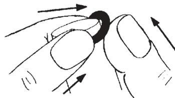
**Figure Q** Ring Removal
