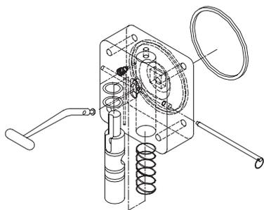
**Figure M** Disassemble Dispensing Valve
