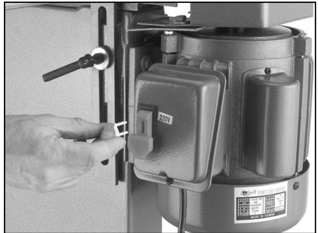
Figure 21. Safety key removed from switch.
