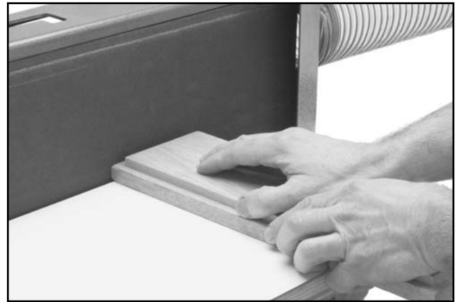
Figure 24. Typical end sanding operation.
