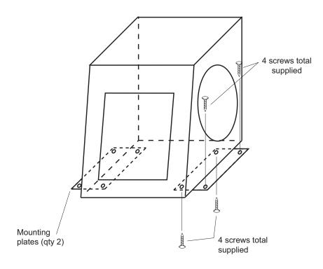
Note: The mounting plates can be installed on any edge of the bottom surface of the subwoofer (shown above mounted on the left and right).
