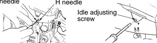
The carburetor on your unit has been factory adjusted, but may require fine tuning due to a change in operating conditions.
