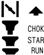
Starting the engine. If you pull out the choke knob (at the back-right of the rear handle) to the point of the arrow, you can set the starting mode as follows:
