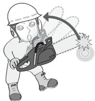
23. Guard against kickback. Kickback is the upward motion of the guide bar which occurs when the saw chain at the nose of the guide bar contacts an object. Kickback can lead to dangerous loss of control of the chain saw.
