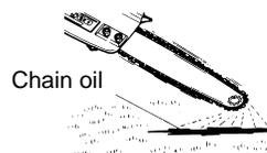
The chain oil flow can be changed by inserting a screwdriver in the hole on bottom of the clutch side. Adjust according to your work conditions.
