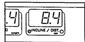
Note: When the INCLINE buttons are pressed, the display will change to show the selected incline setting. If the KPH indicator beside the SPEED display is dark, the distance will be displayed in miles. If the KPH indicator is lit, the distance will be displayed in kilometers.
