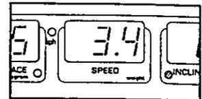
pressed, the speed will change by 0.1 mile per hour (mph). If the buttons are held down, the speed will change in increments of 0.5 mph. The speed range is 0.5 mph to 10 mph. Note: When the SPEED buttons are pressed, the SPEED display will show the selected speed setting for six seconds. The display will then show the actual speed of the walking belt.
