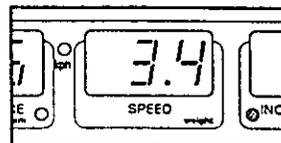
Note: The speed can be shown in either miles per hour (mph) or kilometers per hour (kph). The KPH indicator beside the SPEED display will light when the speed is shown in kph. To change the unit of measurement, first hold down the STOP button while inserting the key into the console. An "E" for English (miles) or an "M" for Metric (kilometers) will appear in the PULSE display. Press the SPEED "+" button to change the unit of measurement. Remove and then reinsert the key.
