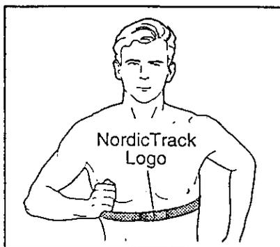
3. Pull the transmitter away from your body a few inches and locate the two electrode areas on the inner side. The electrode areas are the two long, grooved rectangles. Using saline solution such as saliva or contact lens solution, wet both electrode areas. Return the transmitter to a position against your chest.
