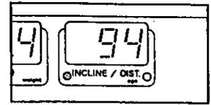
The PULSE display will show an "E," for English (miles), or an "M," for Metric (kilometers). The console will display speed and distance in the unit of measurement shown. Pressing the SPEED "+" button will change the unit of measurement.
