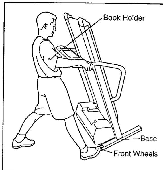
3. Place one foot on the base, and carefully lower the treadmill until it is resting in the storage position.
