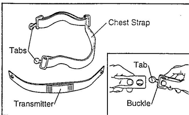
1. Refer to the inset drawing above. Insert the tab on one end of the chest strap through the hole in one end of the transmitter. Press the end of the transmitter under the buckle on the chest strap. The tab should be flush with the front of the transmitter.
