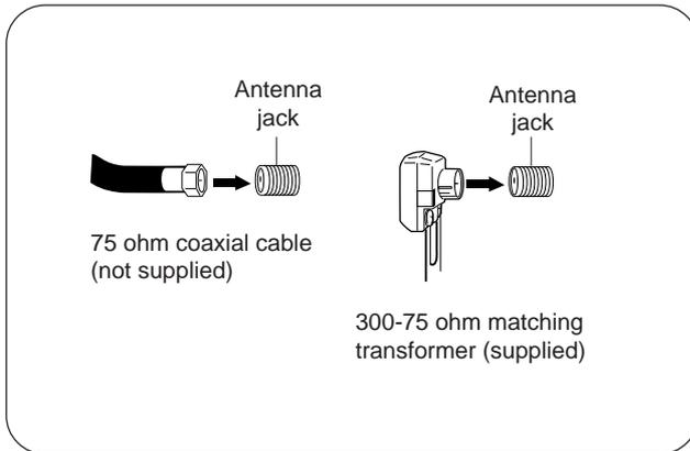
Connect the 75 ohm cable from the combination VHF/UHF antenna to the antenna jack.
