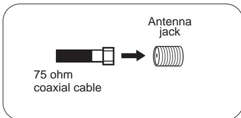
For basic cable service not requiring a converter/descrambler box, connect the Cable TV 75 ohm coaxial cable directly to the Antenna jack on the back of the unit.
