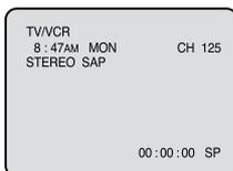
**4 If the clock is not set, check the antenna condition. The Auto clock may not function properly if the reception condition is not good.**
