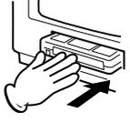
Insert the cassette tape with its labeled side facing up and the erase prevention tab positioned at your left. An inverted cassette tape cannot be inserted.
