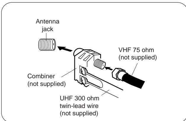
Connect the VHF 75 ohm cable and UHF 300 ohm twin-lead wire to the combiner (not supplied). Attach the combiner to the antenna jack.
