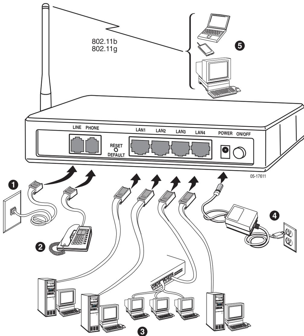
**Figure 2-1. Hardware Installation**
