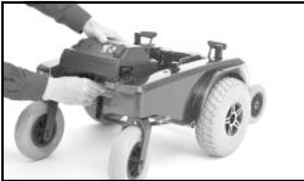
Figure 17. Removing Battery Well Frame
