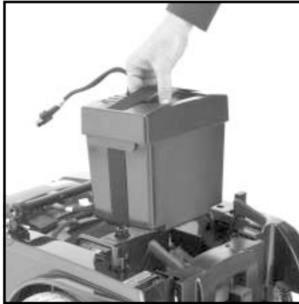
Figure 16. Removing Battery Boxes
