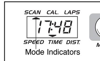
**Speed, time, distance, laps, or calorie mode**—To select one of these modes for continuous display, press the mode button repeatedly. The mode indicators will show which mode is selected. (Make sure that the scan mode is not selected.)
