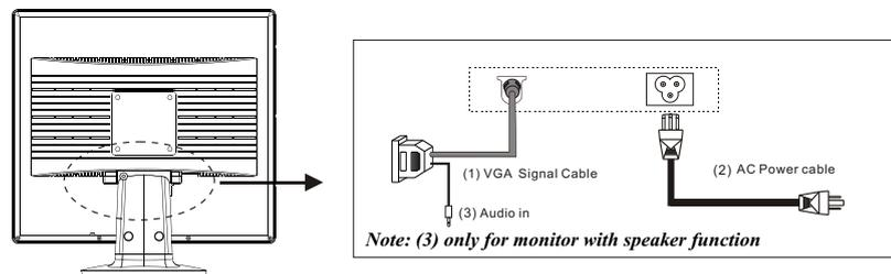
**Connecting the monitor to the computer and the power supply**
