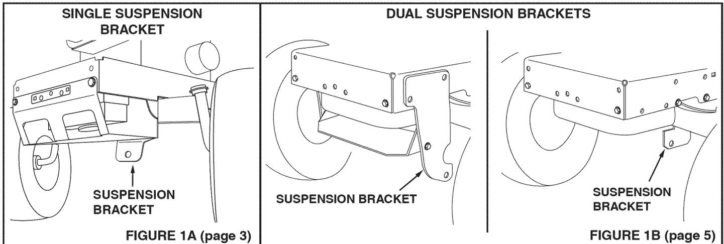
For all tractors with model numbers beginning with 917, look under the front of your tractor (Figure 1A & 1B). If there is a single mower deck suspension bracket located underneath the middle of the front axle, continue on to INSTRUCTIONS FOR SINGLE SUSPENSION BRACKET TRACTORS on page 3. If your tractor does not have a mower deck suspension bracket underneath the middle of the front axle, skip to INSTRUCTIONS FOR DUAL SUSPENSION BRACKET TRACTORS on page 5.
