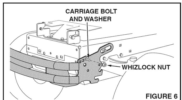
**IMPORTANT:** Before fully tightening nuts, be sure tractor hood will stay in raised position when opened.
