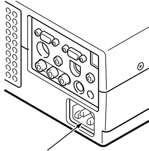
Connect the AC power supply cord (supplied) to the projector. The socket-outlet must be near this equipment and must be easily accessible.
