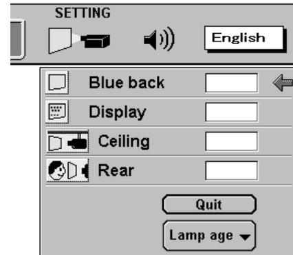
The Lamp age function is designed to reset the lamp
