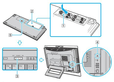
You can check the battery indicator ( or o on the wireless keyboard for its battery power level.
