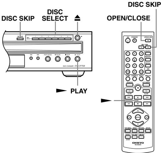
**Tip:** If you press the Play [▶] button, the disc tray will close and playback of the disc in the right bay will start automatically. If there is no disc in that bay, the DV-CP704 will check the other bays and play the first disc it finds.
