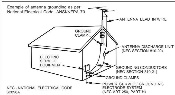
**16 Lightning** - For added protection for this product during a lightning storm, or when it is left unattended and unused for long periods of time, unplug it from the wall outlet and disconnect the antenna or cable system. This will prevent damage to the product due to lightning and power-line surges.
