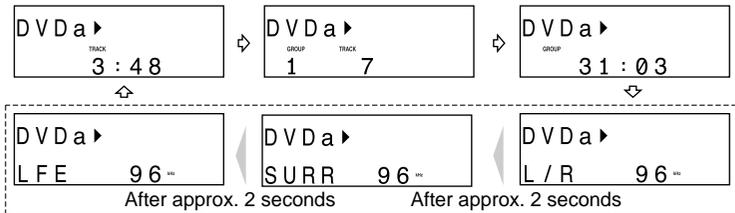
Sampling frequency (low frequency effects)(\*)      Sampling frequency (surround)(\*)      Sampling frequency (2 channel)(\*)
