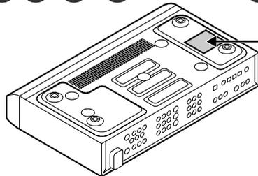
The rating label is located on the bottom of the AV selector.
