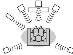
**Dolby Pro Logic II converts 2 channel stereo sound of CDs, etc. to 5.1 channel.**
