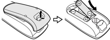
When inserting or removing the batteries, push them toward the  $\ominus$  battery terminals.
