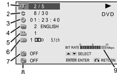
**3** Press the ▲, ▼, ◀ or ▶ button to change the setting and press the ENTER button.
