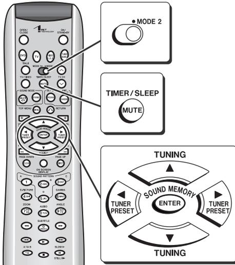
**1** During playback, set the MODE 1/MODE 2 switch to MODE 2 and press the TIMER/SLEEP button.
