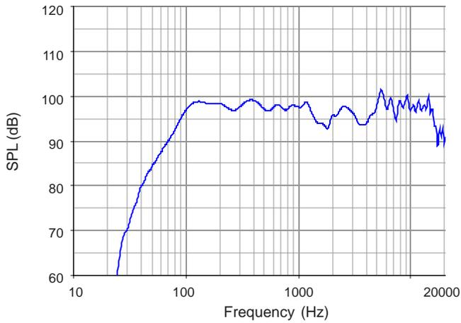
**Frequency Response: Digital Signal Processor**
