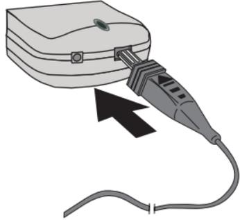
**Note:** DO NOT force the plug as this may damage the phone and/or the charger.
