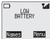
It is recommended that the battery is fully discharged between charges to maintain battery life and performance.
