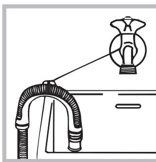
alternatively, rest it on the side of a washbasin or bathtub, fastening the duct supplied to the tap (see figure). The free end of the hose should not be underwater.
