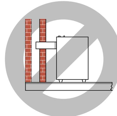
Never extend vent pipe horizontally through a chimney or flue. You must connect a vertical run of vent pipe to the horizontal run. The vertical run must be at least 25% longer or five feet minimum than the horizontal run.
