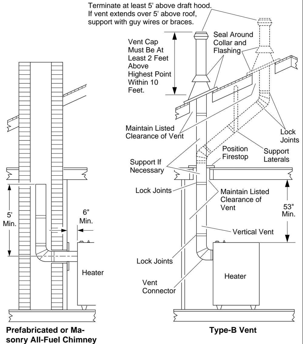
Figure 5 - Typical Construction of Venting Systems
