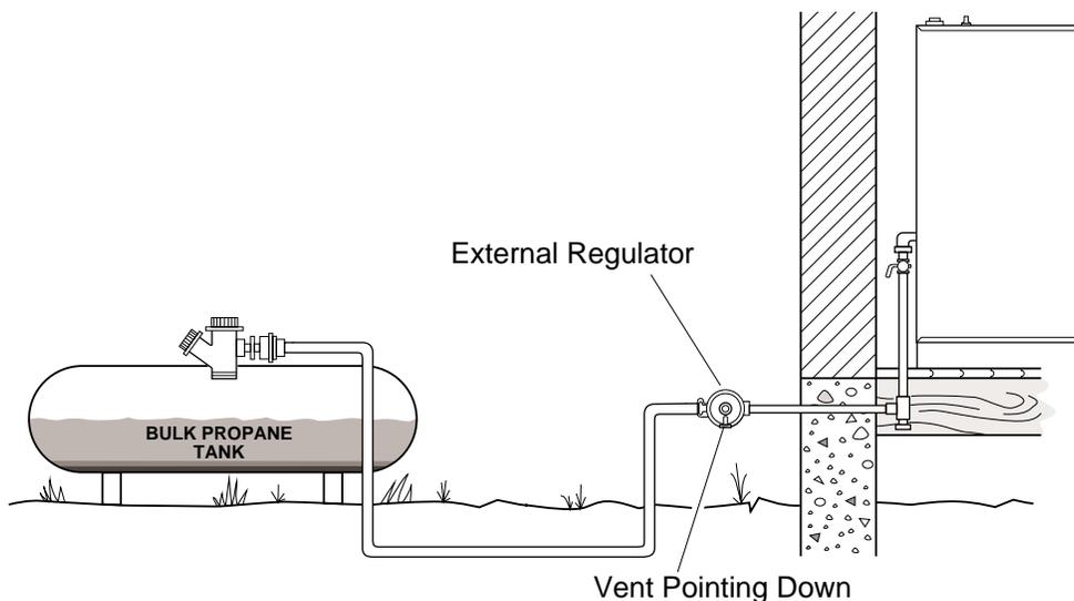
**Figure 6 - External Regulator with Vent Pointing Down**
