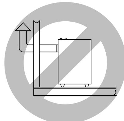
The vertical section of vent pipe must extend at least two feet above the highest point of any roof within ten feet.
