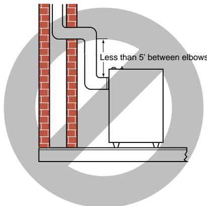
Vertical run of pipe must be at least five feet from elbow to elbow.
