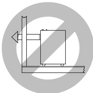
Never extend vent pipe horizontally through outside wall and terminate. You must connect a vertical run of vent pipe to the horizontal run. The vertical run must be at least 25% longer than the horizontal run.
