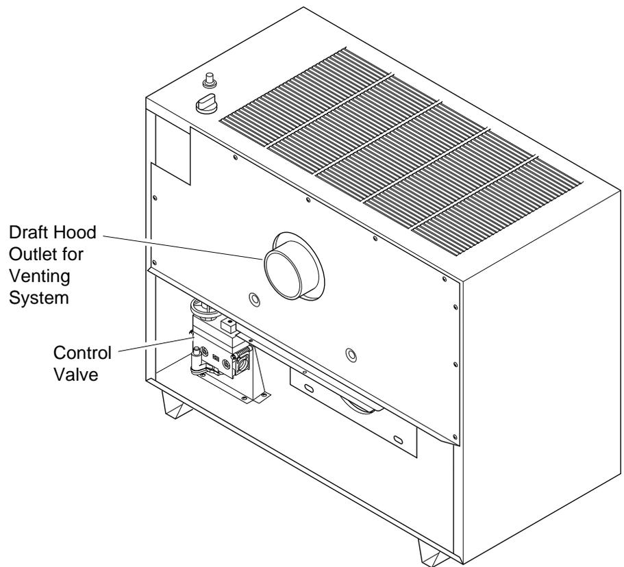
**Figure 2 - Vented Propane Gas Heater, Rear View**
