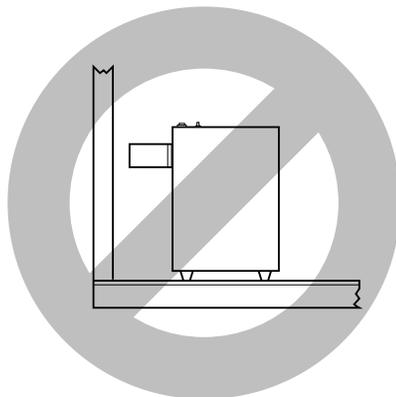
Heater must be vented to the outdoors. Never vent heater to another room or inside a building.
