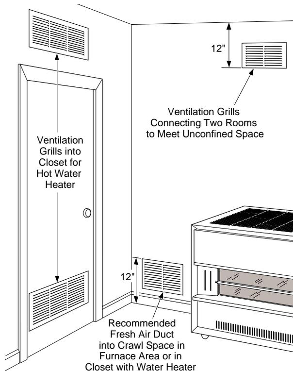
**Figure 15 - Ventilation Air from Inside Building**
