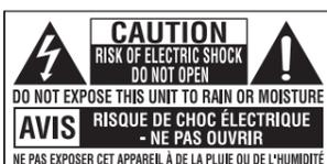
The lightning flash with an arrowhead symbol, within the equilateral triangle, is intended to alert the user to the presence of uninsulated "dangerous voltage" within the product's enclosure that may be of sufficient magnitude to cause an electric shock.
