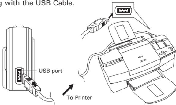
1. USB series A plug connects to the socket marked
