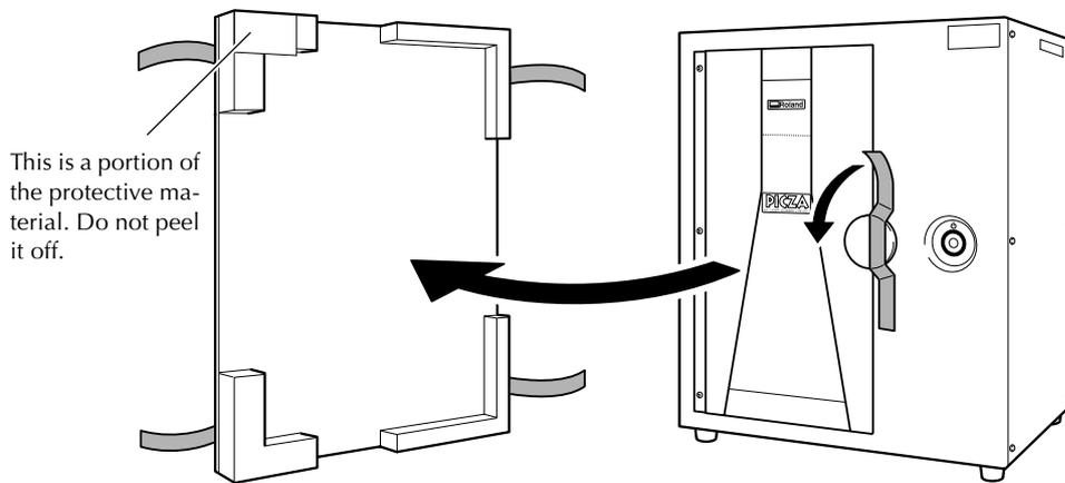
This is a portion of the protective material. Do not peel it off.
