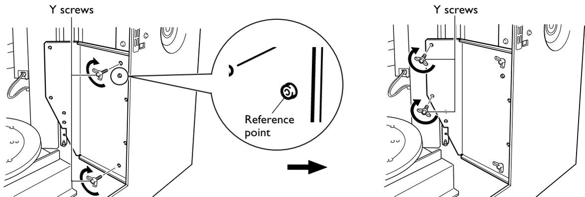
Using the protrusion at the front of the machine as the reference point, provisionally tighten at the front.
