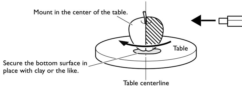
The table rotates during scanning. Using double-sided tape, clay, or the like, fasten the object in place securely so that it will not fall over or slip. Any slipping of the object makes correct scanning impossible.
