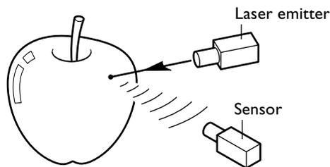
It performs scanning as it rotates the scan object and moves the laser beam from bottom to top.
