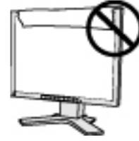
Blocking the ventilation slots prevents proper airflow and may result in fire, electric shock, or equipment damage.
