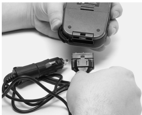
Attach external power cable to iFINDER.
